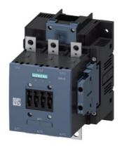
Power contactor, AC-3 150 A, 75 kW / 400 V AC (50-60 Hz) / DC operation 23-26 V UC Auxiliary contacts 2 NO + 2 NC 3-pole, Size S6 Busbar connections Drive: conventional
