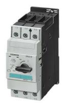
Circuit breaker size S2 for motor protection, Class 10 A-release 22...32 A Short-circuit release 416 A Screw terminal Standard switching capacity !!! Phased-out product !!! Successor is SIRIUS 3RV2 Preferred successor type is >>3RV2031-4EA10<<
