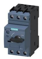
Circuit breaker size S0 for motor protection, CLASS 10 A-release 27...32 A N-release 400 A screw terminal Standard switching capacity
