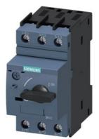
Circuit breaker size S0 for motor protection, CLASS 10 A-release 30...36 A N-release 432 A screw terminal Standard switching capacity
